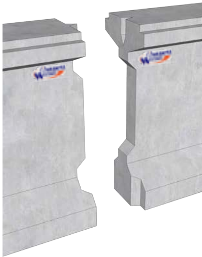
Alt. 1 Shear Key (Match Casting)
